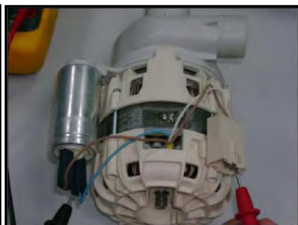
Measurement of the secondary windings of the washing pump ( 126.8 \pm 7\% \Omega )
