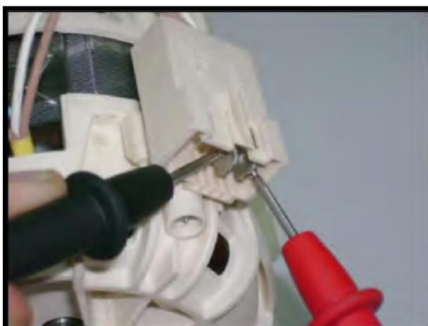
Measurement of the primary windings of the washing pump ( 127.1 \pm 7\% \Omega )
